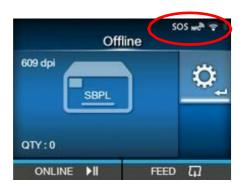
Push the power button on the control panel until the LED lights up in blue and turn on the printer. An initial icon "SOS" is displayed at the top of the printer screen. However the printer is not yet connected with SATO. Please add the printer to your SOS account as following steps..
