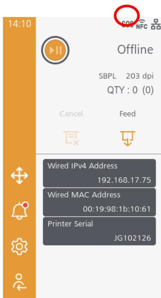
Push the power button on the control panel until the LED lights up in blue and turn on the printer. An initial icon "SOS" is displayed at the top of the printer screen. However, the printer is not yet connected with SOS. Please add the printer to your SOS account as following steps.
