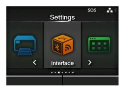
$\cdot$  On the Settings screen for the printer, press the ( $\triangleleft \triangleright$ ) keys to select "Interface", and then press the  $\nleftrightarrow$  key.
