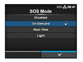
$\cdot$  On the SOS Mode screen, press the ( $\bigtriangleup \nabla$ ) keys to select "On-Demand" or "Light", and then press the  $\overbrace{\cdots}$  key or  $\rightleftarrows$  key.
