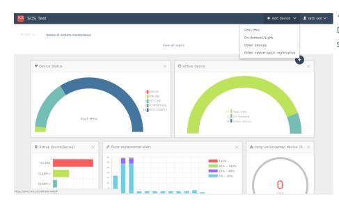
•Click [+ Add device] on the upper right of the Dashboard screen as shown on the left, and select [Other device].
